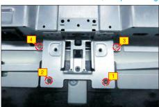
Take away the middle bezel, and put it on a fixture. Use a Philips-head screwdriver to remove 3pcs screws for unlocking the function key board with the middle bezel, and then tear off the tapes for releasing the key cables.
