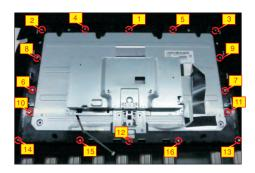
Use a Philips-head screwdriver to remove 2pcs screws for unlocking the bracket chassis with panel module.
