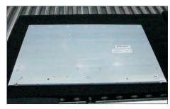
S13 Remove the Mylar from the hooks of the bracket chassis module.
