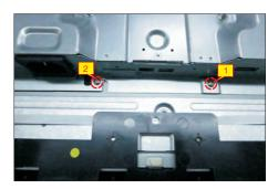
Lift up the middle bezel and take away the middle bezel, and put it on a fixture. Use a Philips-head screwdriver to remove 3pcs screws for unlocking the function key board with the middle bezel, and then tear off the tapes for releasing the key cables.
