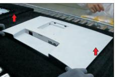
Tear off 2pcs aluminum foils, and then disconnect the function key cable away from the connector of the board. Disconnect the panel lamp cable and function key cable away from the connectors of the panel module and board.
