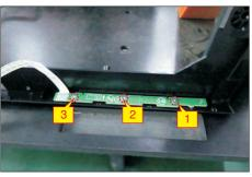
S10 Lift up the panel module with the bracket chassis for releasing the front bezel away from the panel module, and then tear off the tape.
