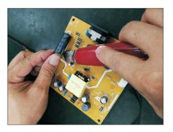
S16-3 Cut into the bottom of bulk cap. and pullit up carefully.
