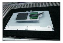
S12 Remove the Mylar from the hooks of the bracket chassis module.
