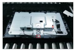
Paste 1pcs aluminum foil to cover the LVDS S14 connector, then paste 1pcs aluminum foil to fix bracket chassis as the picture below shown.
