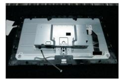
Use a Philips-head screwdriver to tighten 2pcs screws for locking the bracket with middle bezel, to S11 tighten 2pcs screws for locking the bracket with panel.
