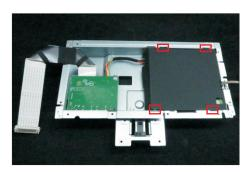
Use a Philips-head screwdriver to remove 5pcs screws for unlocking the circuit board, release all the cables from the hooks.
