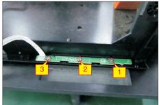
Move the middle bezel with function key board close to the panel unit, tear off the papers of the tapes on the back of the key cable, and then fix the key cable on the bezel by 1pcs tape, then assemble the middle bezel with the front bezel and panel module.
