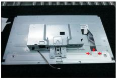
Take away the bracket chassis module and then put the bracket chassis module on a protective cushion.
