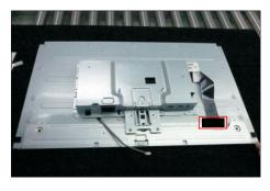
S10 Unplug the LVDS cable from the connector of the panel module by pushing the earing-locks.
