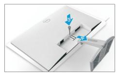
To remove the VESA cover: Press the dimple on the VESA cover to release it from the back of the display.
