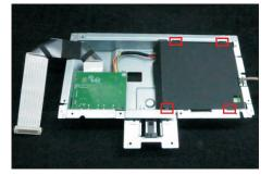
Use a Philips-head screwdriver to remove 5pcs screws for unlocking the circuit board, release all the cables from the hooks.
