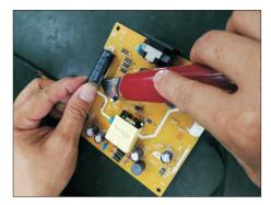
S16-2 Ensure cutting path within the glue, don't touch bulk cap. or PCB.
