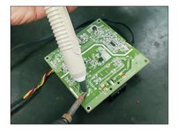
S16-5 Lift the bulk cap. up and away from the PCB.
