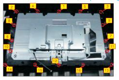
Use a Philips-head screwdriver to remove 2pcs screws for unlocking the bracket with middle bezel, to remove 2pcs screws for unlocking the bracket with panel module.
