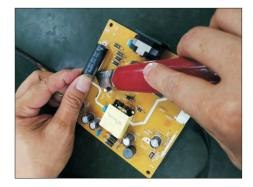
S16-3 Cut into the bottom of bulk cap. and pullit up carefully.
