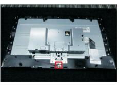
Take a pair of speakers to locate the probers of the middle bezel, then connect the speaker cable to the connector of the board. Paste 1pcs aluminum foil to fix the bracket on the specific position.
