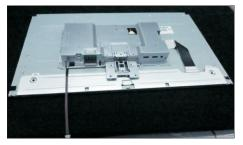
Paste 1pcs tape to cover the LVDS connector. Take1pcs front bezel, then lift up the panel with bracketand assemble the front bezel with the panel module.
