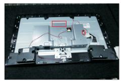
Use a Philips-head screwdriver to tighten 6pcs screws for locking the speakers with middle bezel. Settle the cable and then fix the speaker's cables with 2pcs acetate tapes on the specific position as the picture below shown.
