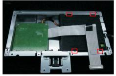
Panel preparation: Take out 1pcs panel module from the carton, then remove the protective film by tearing off the tapes, and then examine the panel surface according to inspection criteria. Turn over the panel, and then place screen faced down for later assembling.
