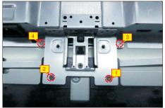
Take away the middle bezel. Use a Philips-head screwdriver to remove 3pcs screws for unlocking the function key board with the middle bezel, and then tear off the tapes for releasing the key cables. (No.1~3 screw size=M2x2.4, Torque=0.8±0.2kgfxcm
