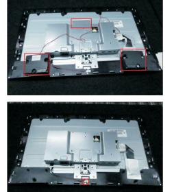
Use a Philips-head screwdriver to remove 16pcs screws for unlocking the middle bezel. (No.1~11 screw size=M3x4, Torque=3~4kgfxcm; No.12~16 screw size=M2x3.3, Torque=1±0.2kgfxcm)
