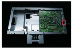
Take a interface board, connect a LVDS cable to the connector of the interface board, then connect the cable of the power board to the connector of the interface board. Turn over the interface board and locate it into the bracket. Use a Philips-head screwdriver to tighten six screws for locking the power board and interface board.
