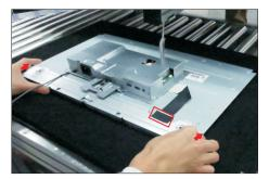
Take a function key board and a middle bezel, then fix the middle bezel with a fixture, and locate the function keyboard into the hooks of the bezel. Use a Philips-head screwdriver to tighten 3pcs screws for locking the function key board with the middle bezel. (No.1~3 screw size=M2x2.4, Torque=0.8±0.2kgfxcm
