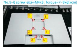
Stick 2pcs labels on the specific positions as the picture below shown. Take 1pcs stand riser and 1pcs stand base, assemble the stand base with stand riser, then rotate the screw clockwise to lock the stand base and stand riser. Insert the stand-riser into monitor groove until it snaps into its place.
