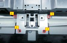
S12 Connect the function key cable to the connector of board, then paste 1pcs aluminum foil to cover the LVDS connector and key cable.
