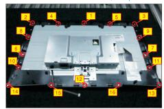
Tear off 1pcs aluminium foil, and then disconnect the function key cable away from the connector.
