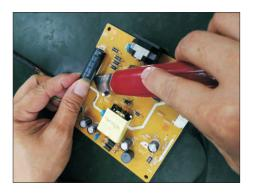
S18-4 Take out bulk cap. pin solder with soldering iron and absorber.
