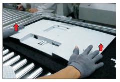
Tear off 2pcs acetate tapes and then disconnect the speaker cable away from the connector. Use a Philips-head screwdriver to remove 6pcs screws for unlocking the speakers with middle bezel.
