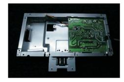
S17 Remove the interface board and power board from the bracket chassis module carefully, and disconnect all the cables.
