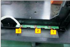
Tear off the tape, then lift up the panel module with the bracket chassis for releasing the front bezel away from the panel module.
