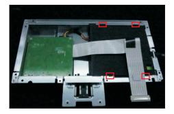
Use a Philips-head screwdriver to remove six screws for unlocking the circuit board, release all the cables from the hooks.
