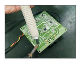
S19-5 Lift the bulk cap. up and away from the PCB.
