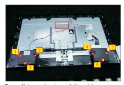
Tear off 1pcs aluminum foil and then remove the two speakers. Disconnect the panel lamp cable away from the connector of the panel module.
