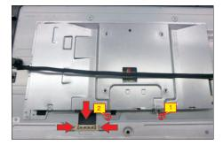
Use a Philips-head screwdriver to remove 13pcs screws for unlocking the middle bezel with the assembled unit.
