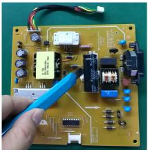
S1 -3 Cut into the bottom of bulk cap. and pull it up carefully
