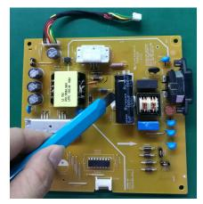
S1 -2 Ensure cutting path within the glue, don't touch bulk cap. or PCB
