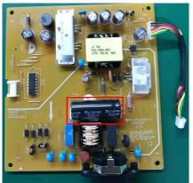
S1 -1 Cut the glue between bulk cap. and PCB with a knife
