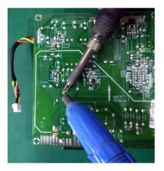
S1 -5 Lift the bulk cap. up and away from the PCB
