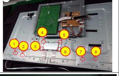
Use a Philips-head screwdriver to remove 8 screws for remove BKT (No.1~8 screw size=M3x6; Torque=4±1kgf.cm)
