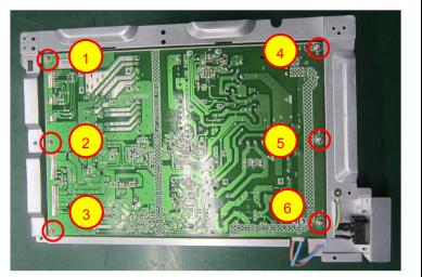
Use a Philips-head screwdriver to remove 11 screws for Remove Main board and Inverter board (No.1~11 screw size=M3x6; Torque=6±1kgf.cm)
