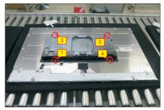
Move up the bracket, then disconnect the EDP cable away from the connectors of the panel module.
