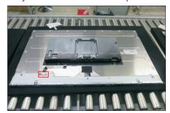
S17 Remove the bracket and put it on a cushion. Lift up the panel for releasing the front bezel away from the panel. Tear off the acetate tape.
