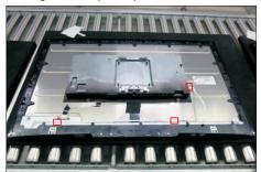
Take away the middle bezel, and put it on a fixture, then tear off the mylar tape for releasing the LED board.
