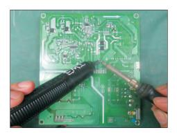
S21-5 Lift the bulk cap. up and away from the PCB.
