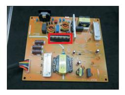
S21-1 Cut the glue between bulk cap. and PCB with a knife.
