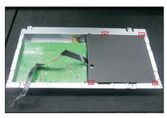
Use a Philips-head screwdriver to remove 7pcs
