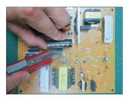
S21-2 Ensure cutting path within the glue, don't touch bulk cap. or PCB.
