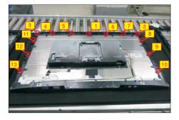
Use a Philips-head screwdriver to remove 2pcs screws for unlocking the middle bezel with the front bezel. Disconnect the panel lamp from the connectors of the panel and board.
