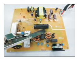
S20-4 Take out bulk cap. pin solder with soldering iron and absorber.
