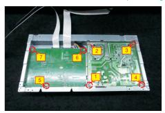
S20 Remove the power board board and interface board from the bracket chassis module carefully, and then disconnect all of the cables.
