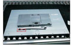
S17 Take away the bracket chassis module and then put the bracket chassis module on a protective cushion.
