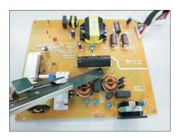
S20-3 Cut into the bottom of bulk cap. and pullit up carefully.
