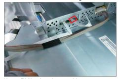
Use a Philips-head screwdriver to remove 2pcs screw for unlocking the key board, then tear off the tapes and release the key board.
