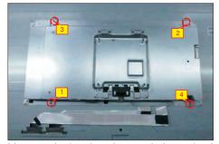
Move up the bracket, then push the earing-lock and disconnect the 2pcs LVDS cables away from the connectors of the panel module.
