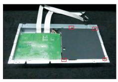
Use a Philips-head screwdriver to remove 7pcs screws for interface board and power board.
