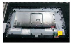
Disconnect the panel lamp cable away from the connectors of the panel module and circuit board, then release the cable by tearing off tape.
