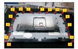
S11 Disconnect the LED cable from the connector of the board, then tear off 3pcs aluminum foil.
