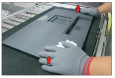
Lift the rear cover up carefully. Disconnect the key cable and USB FFC cable from the connectors of the interface board, and then remove the rear cover.
