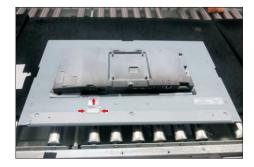
Take away the bracket chassis module and then put S16 the bracket chassis module on a protective cushion.
