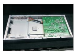
Remove the interface board and power board from S19 the bracket chassis module carefully, and disconnect all the cables.
