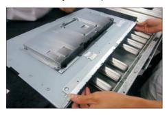
Use a Philips-head screwdriver to remove 2pcs \$14 screws for unlocking the bracket with panel module. (No.1~2 screw size=M3x4, Torque=5±0.5kgfxcm)
