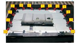
Disconnect the LED cable from the connector, then release the LED cable by tearing off the tapes. Tear S11 off the acetate tape, and then release the panel lamp cable from the hook of the middle bezel.
