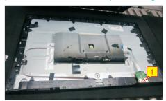
Tear off 2pcs aluminium foils and 1pcs conductive tape for unfixing the bracket. Use a Philips-head screwdriver to remove 2pcs screws for locking the middle with the front bezel and the panel.
