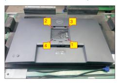
Wedge your fingers between the rear cover and the middle bezel on the corners of the top side of the monitor to release the rear cover, then use one hand to press the middle bezel, the other hand to pull up carefully the rear cover in order of arrow preference for unlocking mechanisms of rear cover.
