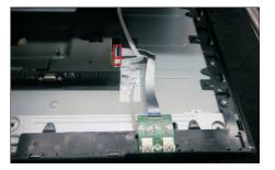
Use a Philips-head screwdriver to remove 2pcs screws for unlocking the joystick key board unit, then **S7** tear off the tapes and release the USB board.
