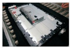
Take away the middle bezel, and put it on a fixture, S12 then tear off the mylar tape for releasing the LED board.
