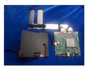
Hold the plastic button on the power board to separate the Mylar from the power board.
