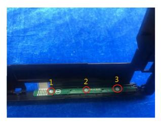
Use a Philips-head screwdriver to remove 1 screws to remove the USB board. Disconnect the cables of the USB board
