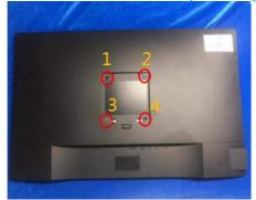
Wedge your fingers between the rear cover and the middle bezel on the corners of the top side of the monitor to release the rear cover, then use Scraper
