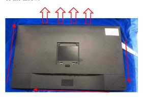
Tear out all the cable to remove the rear cover and put it on a protective cushion. Use a Philips-head screwdriver to remove 11 screws for unlocking the middle plastic bezel with the whole unit, and then remove the middle plastic bezel carefully.
