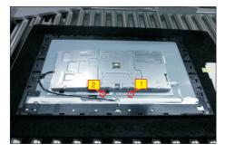
Release the panel lamp cable from the hook of the middle bezel. Use a proper tool to release the function key cable from the connector, then pull the function key cable high for releasing the function key cable.
