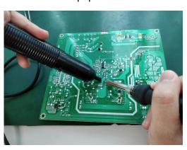
S19-5 Lift the bulk cap. up and away from the PCB
