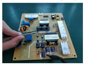
S19-4 Take out bulk cap. pin solder with soldering iron and absorber
