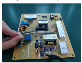
S19-2 Ensure cutting path within the glue, don't touch bulk cap. or PCB
