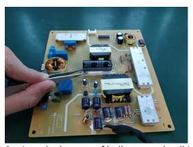
S19-3 Cut into the bottom of bulk cap. and pull it up carefully
