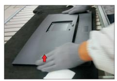
Lift the rear cover up carefully. Disconnect the USB FFC cable from the connector of the interface board, and then remove the rear cover.
