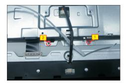
Use a Philips-head screwdriver to remove 15pcs screws for unlocking the middle bezel with the assembled unit.
