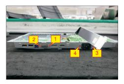
Remove the Mylar from the hooks of the bracket.
