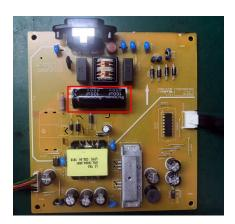
S19-1 Cut the glue between bulk cap. and PCB with a knife
