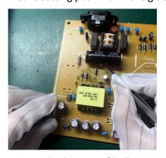
S19-3 Cut into the bottom of bulk cap. and pull it up carefully
