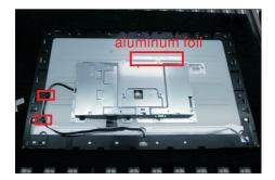
Use a Philips-head screwdriver to remove 2pcs screws for unlocking the bracket with the panel.
