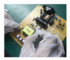
S19-4 Take out bulk cap. pin solder with soldering iron and absorber
