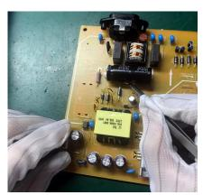
S19-2 Ensure cutting path within the glue, don't touch bulk cap. or PCB
