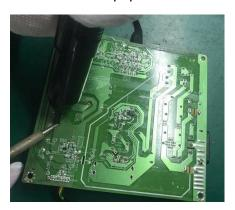
S19-5 Lift the bulk cap. up and away from the PCB
