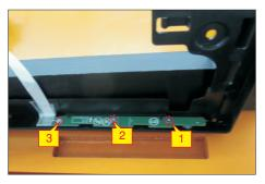
S13 Lift up the panel module with the bracket chassis for releasing the front bezel away from the panel module.
