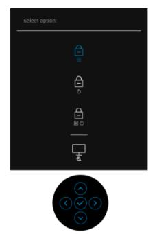
**3.** Move the joystick to highlight the Diagnostic icon and then press the joystick to confirm. A gray test pattern appears.
