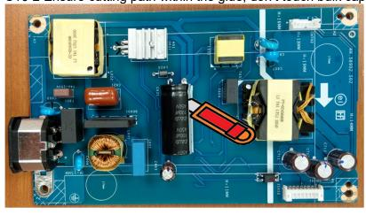
S16-3 Take out bulk cap. pin solder with soldering iron and absorber
