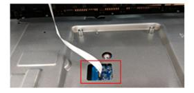
S5 Tear off 1 tape from CTRL BD FFC on Rear Cover
