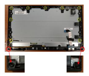
(Screw Torque-MF: 3.5~~4.0kgf) (Screw Torque-BZL Chin: 2.0±0.1kgf)
