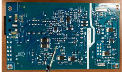
S16-4 Lift the bulk cap. up and away from the PCB
