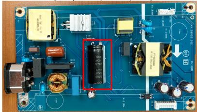
S16-1 Cut the glue between bulk cap. and PCB with a knife
