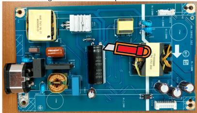
S16-2 Ensure cutting path within the glue, don't touch bulk cap. or PCB
