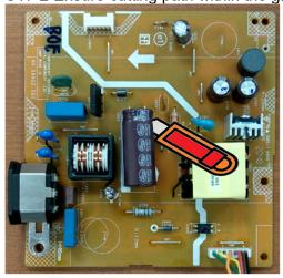
S17-3 Take out bulk cap. pin solder with soldering iron and absorber
