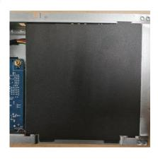
S14 Unlock 5 PCB screws and 2 hex screws
