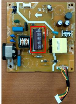
S17-1 Cut the glue between bulk cap. and PCB with a knife
