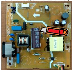
S17-2 Ensure cutting path within the glue, don't touch bulk cap. or PCB
