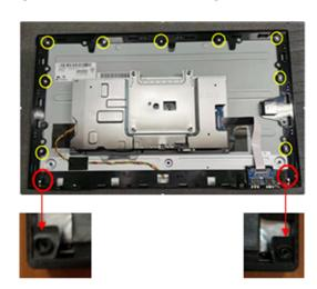
(Screw Torque-MF: 3.5~~4.0kgf) (Screw Torque-BZL Chin: 2.0±0.1kgf)
