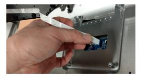
S5 Tear off 1 tape from CTRL BD FFC on Rear Cover
