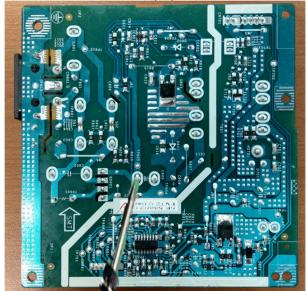
S17-4 Lift the bulk cap. up and away from the PCB
