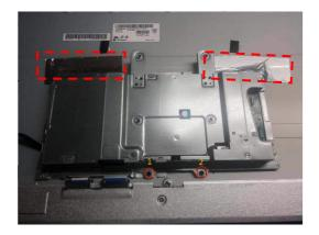
Use a Philips-head screwdriver to remove 7 screws for unlocking the main board and the adapter board
