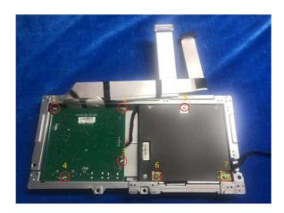
Disconnect all of the cables to separate the power board and main board.
