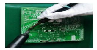
Lift the bulk cap up away from the PCB.
