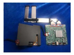
Hold the plastic button on the power board to separate the Mylar from the power board.
