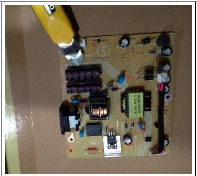
Lift the bulk cap. up and away from the PCB
