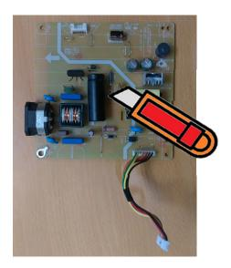
S14-2 Ensure cutting path within the glue, don't touch bulk cap. or PCB
