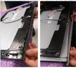
S11 Disassemble Mylar from Main Shielding
