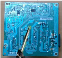
S14-4 Lift the bulk cap. up and away from the PCB
