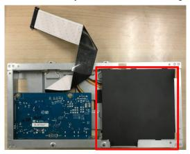
S12 Unlock 6 PCB screws and 2 hex screws
