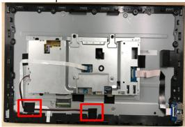
Pull out USB board cable from USB Board and I/F Board
