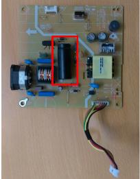
S14-1 Cut the glue between bulk cap. and PCB with a knife
