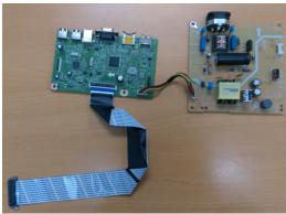
S14 Remove electrolyte capacitors (red mark) from printed circuit boards
