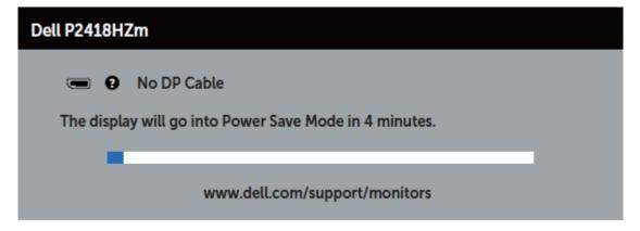
**NOTE:** This box also appears during normal system operation, if the video cable is disconnected or damaged.
