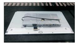
S14 Lift up the panel module for releasing the front bezel away from the panel module.
