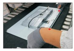
S15 Take away the bracket chassis module and then put the bracket chassis module on a protective cushion.
