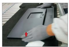
Lift the rear cover up carefully. Disconnect the USB FFC cable from the connector of the interface board, and then remove the rear cover.
