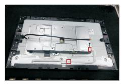
Use a Philips-head screwdriver to remove 2pcs screws for unlocking the bracket with the panel. Push the earing-lock, and disconnect the LVDS cable from the connector of LCD panel module. (No.1~2 screw size=M3x2.8, Torque=2~3kgfxcm)
