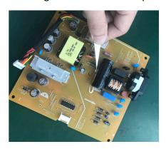
S1 -2 Ensure cutting path within the glue, don't touch bulk cap. or PCB
