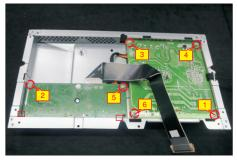
Remove the interface board and power board from the bracket chassis module carefully, and disconnect all the cables.
