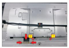
Use a Philips-head screwdriver to remove 13pcs screws for unlocking the middle bezel with the assembled unit.
