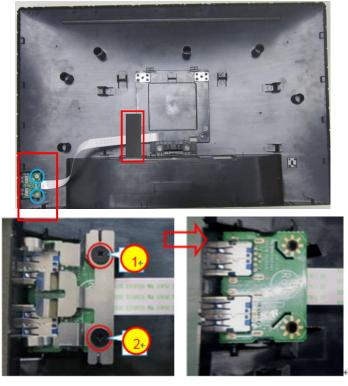
Use a Philips-head screwdriver to remove 2 screws for unlocking USB board.
