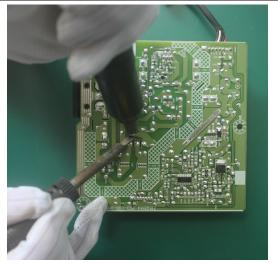
Take out bulk cap. pin solder with soldering iron and absorber
