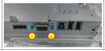
Use a hex screwdriver to remove 2 screws for unlocking mainboard (No.1~2 Hex screw Torque= 4.5± 0.5kgf.cm)
