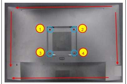
Use a Philips-head screwdriver to remove 4 screws for unlocking mechanisms.
