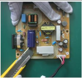
Lift the bulk cap. up and away from the PCB
