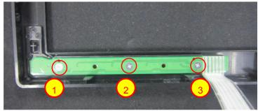
Use a Philips-head screwdriver to remove 3 screws for unlocking key board (No.1~3 screw size=M2x2.5; Torque=0.9±0.4kgf.cm)
