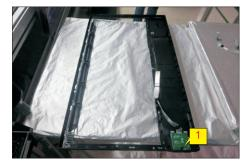
Tear off the two pieces of PVC tape, then disconnect the two panel power cables away from the connectors of the panel module, then release the panel power cable by tearing off the adhesive tapes.
