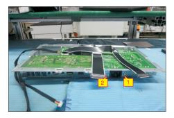
Use a Philips-head screwdriver to remove seven screws for unlocking interface board, LED driver board and power board, then release the panel power cable by tearing off the adhesive tape. (No.1 screw size=M4x8, Torque=7~8kgfxcm; No.2~7 screw size=M3x7.5, Torque=7~8kgfxcm)
