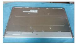
Turn over the bracket chassis module. Remove the Mylar from the hooks of the bracket, and then use a Philips-head screwdriver to remove two screws for
