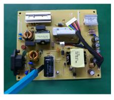
S1 -3 Cut into the bottom of bulk cap. and pull it up carefully
