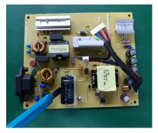
S1 -2 Ensure cutting path within the glue, don't touch bulk cap. or PCB
