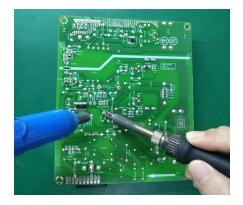
S1 -5 Lift the bulk cap. up and away from the PCB
