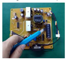
S17-2 Ensure cutting path within the glue, don't touch bulk cap. or PCB
