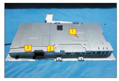
Turn over the bracket chassis module. Remove the Mylar from the hooks of the bracket, and then use a Philips-head screwdriver to remove two screws for unlocking AC power outlet.
