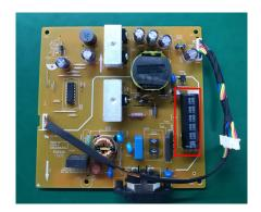
S17-1 Cut the glue between bulk cap. and PCB with a knife
