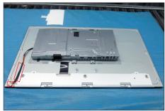
S13 Push the earing-lock and disconnect the LVDS cable away from the connector of the panel module.
