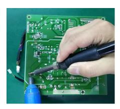
S17-5 Lift the bulk cap. up and away from the PCB
