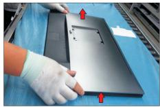
Remove the rear cover. Tear off the aluminum foil, and then disconnect the USB cable away from the connector of the circuit board. Use a a Philips-head screwdriver to remove one screw for unlocking the USB unit, remove the USB unit from the hooks.
