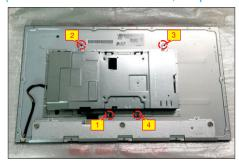
Release the panel cable by tearing off the adhesive tape, and then disconnect the panel power cable away from the connector of the panel module.
