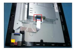
Use a Philips-head screwdriver to release 12 screws for unlocking the middle bezel with the assembled unit.
