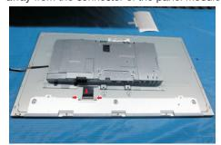
S14 Lift up the bracket chassis module and put it on a protector cushion.
