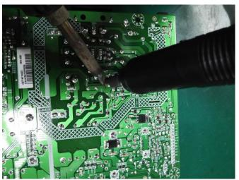
Take out bulk cap. pin solder with soldering iron and absorber
