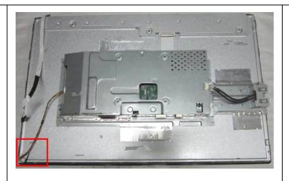
S7. Remove the TAPE and panel FFC cable
