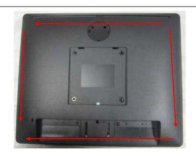
Use Penknife to separate the bezel and rear cove follow the arrows in sequence, then you can take out rear cover.
