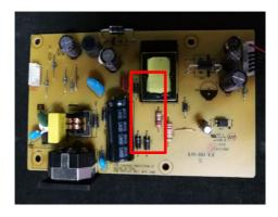
a. Take out the capacitor pin solder with soldering iron.
