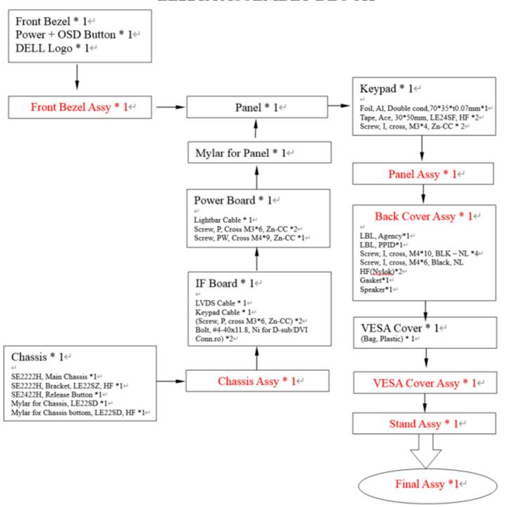
Note: 1. The arrows point out the direction of disassembly. **Disassemble the slot of Back cover from monitor**
