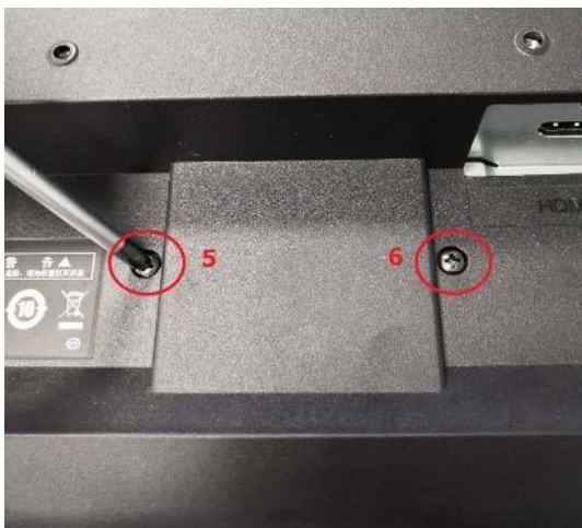
(No.1-4 screw size=M4x12; Torque=7.5-8.5kgfxcm No.5-6 screw size=M3x6; Torque=5-6kgfxcm.)
