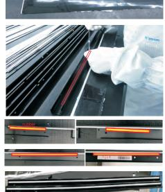
Take 1pcs light pipe, and then use a screwdriver to lock 2pcs screws for locking the light pipe with front bezel. Take 1pcs IR board and 1pcs IR holder and 1pcs shading tape, then assemble the IR board with IR holder, then use a screwdriver to lock 2pcs screws for locking the IR holder with front bezel, then assemble 1pcs IR board cover to bottom-side bezel.
