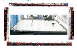
Use a screwdriver to remove 15pcs screws for unlocking H-beam with the assembled unit, and then remove the H-Beam.
