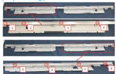
Tear off 16pcs acetate tapes, then use a screwdriver S19 to remove 17pcs screws for unlocking the bottommiddle bezel.(Torque: 3.5±0.3kgf)
