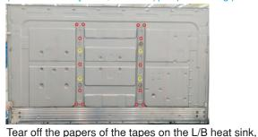
then assemble the L/B heat sink with back bracket.
