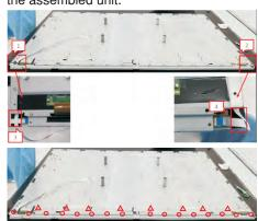
Remove all the bezel and strips and put them on a protective cushion. Open the IR board cover, then use a screwdriver to remove 2pcs screws for unlocking the IR board and holder with front bezel, then use a screwdriver to remove 2pcs screws for unlocking the light pipe with front bezel. (Torque: 3±0.3kgf)
