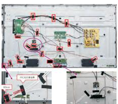
Place 1pcs PC box to the specific positions of the whole unit, then use a screwdriver to lock 7pcs screws for fixing the PC box. (Torque: 4.5±0.3kgf)
