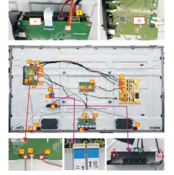
S6 Use a screwdriver to remove 8pcs screws for unlocking the two speakers. (Torque: 4.5kgf±0.5)
