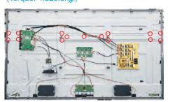
S12 Disconnect the touch cable and FFC cables. Use a screwdriver to remove 24pcs(16+8) screws
