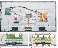
Use a screwdriver to lock 4pcs screws to the back bracket, then use a screwdriver to lock 4pcs screws for locking 1pcs main board with the screws, and then assemble 1pcs USB board and 1pcs IO holder with the main board, then lock 4pcs screws for locking the USB board, lock 2pcs hex screws for locking the VGA connectors. (Torque:4.5kgf±0.5)
