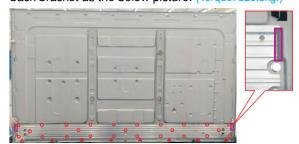
Tear off the papers of double-faced tapes on the L/B, then paste 3pcs L/B from left to right on the hooks of the L/B heat sink, then use a laminating fixture to fix the light bar with the heat sink.
