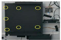
Paste 1pcs for fixing the cable as the picture below shown. Remove 16pcs acetate tapes(size: 80mm) and 1pcs acetate tapes(size: 60mm) for unfixing the cables as the picture below shown.
