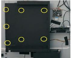
Take 1pcs rear cover, assemble the rear cover with the assembled unit, then use a screwdriver to lock the rear cover with 69pcs screws.(Torque: 3±0.3kgf)
