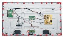
Use a screwdriver to remove 2pcs screws for unlocking the key board and the holder with strip. (Torque: 2±0.3kgf)
