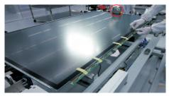
Tear off the tape of SB of O/C, paste 4pcs foams on the SB, then paste 2pcs long foams on the back bracket. Tear off the release tapes and paste the SB on the back bracket, then paste 16pcs conductive foams on the COF of the SB. Use the tipper to turn over the unit to let the back bracket faced up.
