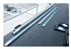
Place the Top, left, right and bottom assembled ED holder units to form a square and then connect them with the FFC cables, then fix the ED unit with a fixture. Connect the FFC cable of ED board to the connectors of the touch board, then connect the power cable and signal cable to the touch board, then run the special program and input SN for testing, it stand ok when you see Pass on the screen.
