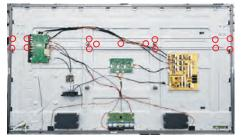
Assemble 4pcs front bezels(top, left, right, bottom) with the assembled unit, then use a screwdriver to tighten 38pcs screws for locking the front bezels with the assembled unit.(Torque: 3±0.3kgf)
