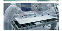
Place 1pcs Diffuser film on the back bracket, then
