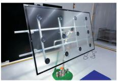
Use a sucking tool to suck the glass and then assemble the glass with the O/C module, then tear off all release papers around edges of the O/C module., and then press the glass with a roll for two parts firmly attachment.
