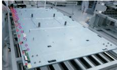
Tear off 12pcs conductive foams on the specific position of the O/C SB, then release the O/C SB away from the back bracket.
