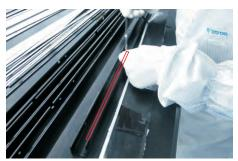
Take 1pcs light pipe, and then use a screwdriver to lock 2pcs screws for locking the light pipe with front bezel. Take 1pcs IR board and 1pcs IR holder and 1pcs shading tape, then assemble the IR board with IR holder, then use a screwdriver to lock 2pcs screws for locking the IR holder with front bezel.(Torque: 3±0.3kgf)
