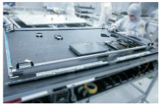
Use a screwdriver to remove 24pcs screws for unlocking the bottom-middle bezel and then remove the bottom-middle bezel.(Torque: 2±0.3kgf)
