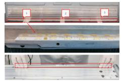
Assemble 2pcs fixture rubber on the side of the back bracket, then place 1pcs Reflector film into the back bracket. Make sure the gap between light and Reflector >1.2mm.
