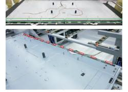
Make sure ED FFC cables are connected well, then assemble 1pcs ED holder with the assembled unit, and then use a screwdriver to tighten 13pcs screws for locking the ED holder with the assembled unit. (Torque: 6±0.3kgf)Use a screwdriver to tighten 12pcs screws for locking the ED holder with the unit. (Torque: 3±0.3kgf)
