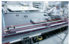
Assemble the ED holders unit with the assembled back bracket, then push the whole unit into a tripper, then fix the FFC cables with tapes, then paste 2pcs rubbers on the specific position as the picture below shown.
