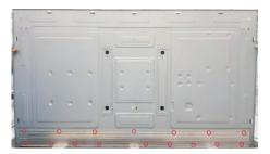
Use a screwdriver to remove10pcs screws for unlocking the two VESA brackets with back bracket.(Torque: 5±0.3kgf)
