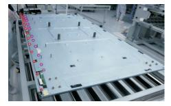
Take 1pcs touch cable to connect the ED boards as picture 1. Take 1pcs folded FFC cable to connect the S25 ED boards as picture 2, then assemble 2pcs rubbers to the assembled unit as picture 3 and picture 4.
