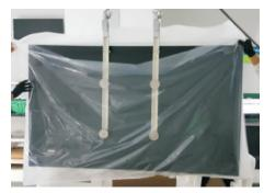
Use a screwdriver to remove 8pcs screws for releasing the handles. (Torque:15±0.5kgf).
