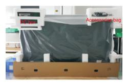
Take out 3pcs desiccant from the bag. Use a machine jip to take out the whole monitor from the EPS-bottom. Remove the PE bag from top to bottom, and put the monitor on ESD protection foam.
