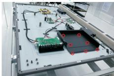
Remove 2pcs O/C mylar tapes away from the back bracket, then remove 22pcs black tapes and 1pcs conductive tape as the picture below shown.
