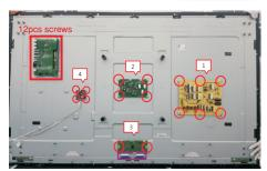
Use a screwdriver to remove 42pcs screws
