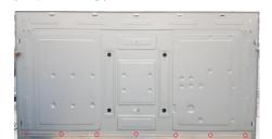
Use a screwdriver to remove10pcs screws for unlocking the two VESA brackets with back bracket.(Torque: 5±0.3kgf)
