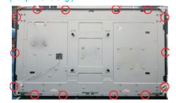
Disconnect the touch cable and FFC cables. Use a screwdriver to remove13pcs screws(Torque: 6±0.3kgf), 12pcs screws (Torque: 3±0.3kgf) for unlocking the ED holder with the assembled unit.
