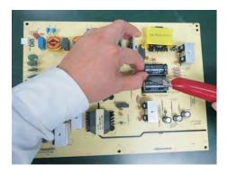
S25-3 Cut into the bottom of bulk cap. and pullit up carefully.
