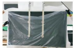
Use a screwdriver to remove 8pcs screws for releasing the handles. (Torque:15±0.5kgf)
