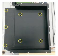
Tear off 1pcs conductive tape for releasing main board, USB board and LVDS cable. Remove 2pcs white mylar tapes.
