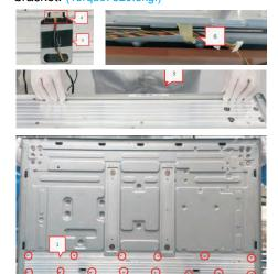
Use a screwdriver to remove10pcs screws for unlocking the two VESA brackets with back bracket.(Torque: 5±0.5kgf)
