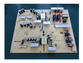
S12-1 Cut the glue between bulk cap. and PCB with a knife
