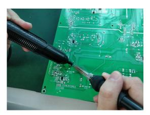
S12-5 Lift the bulk cap. up and away from the PCB
