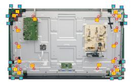
Remove the 4pcs conductive tapes and 8pcs rubbers. Use a screwdriver to remove 12pcs screws for unlocking the side iron. (Torque: 3.8kgf±0.3) Remove 1pcs PVC tape. Remove the main board, touch board with cables and power board.
