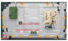
S10 Lift up the assembled ED unit. Lift up the panel module with a proper tool and put it on a protective cushion. Lift up the glass with a tool and put it on a protector.
