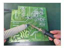
S22-5 Lift the bulk cap. up and away from the PCB.
