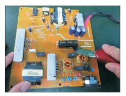
S22-2 Ensure cutting path within the glue, don't touch bulk cap. or PCB.
