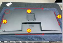
Lift the rear cover up carefully. Disconnect the joystick key cable and two USB cables from the connectors of the board, and then remove the rear cover and put it aside for later disassembling.
