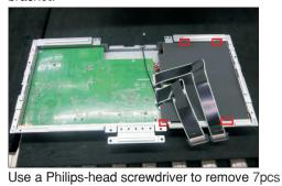
screws for interface board and power board.
