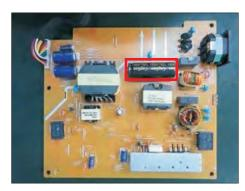
S24-1 Cut the glue between bulk cap. and PCB with a knife.
