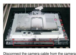
board, and then Use a Philips-head screwdriver to remove 4pcs screws for unlocking the camera module with the middle bezel, to remove 4pcs screws for unlocking the bracket.
