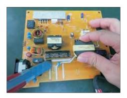
S24-2 Ensure cutting path within the glue, don't touch bulk cap. or PCB.
