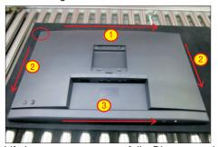
S7 Lift the rear cover up carefully. Disconnect the joystick key cable and two USB cables from the connectors of the board, and then remove the rear cover and put it aside for later disassembling.
