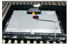
Tear off the camera glass and tape of the camera connective cable, then use a Philips-head screwdriver to remove 2pcs screws for unlocking the rear cover with front cover, and then disassemble the rear cover of camera from the unit, and then tear off the camera from the front bezel.
