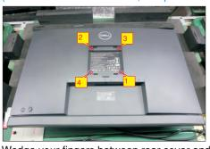
Wedge your fingers between rear cover and the middle bezel on the corners of the top side of the monitor to release the rear cover, then use one hand to press the middle bezel, the other hand to pull up carefully the rear cover in order of arrow preference for unlocking mechanisms of rear cover.
