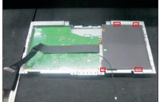
Use a Philips-head screwdriver to remove 7pcs screws for interface board and power board.
