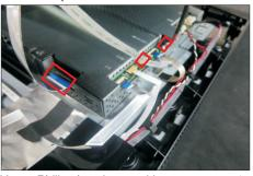
Use a Philips-head screwdriver to remove 1pcs screw for unlocking the USB board, then tear off all the tapes and release the Usb power cable and joystick cable.
