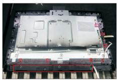
Use a Philips-head screwdriver to remove 2pcs screws for unlocking the camera module with the middle bezel, to remove 4pcs screws for unlocking the bracket with the panel module.
