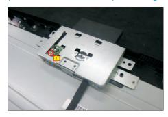
Tear off the camera glass and tape of the camera connective cable, then use a Philips-head screwdriver to remove 2pcs screws for unlocking the rear cover with front cover, and then disassemble the rear cover of camera from the unit, and then tear off the camera from the front cover.
