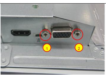
Use a hex screwdriver to remove 2 screws for unlocking mainboard.
