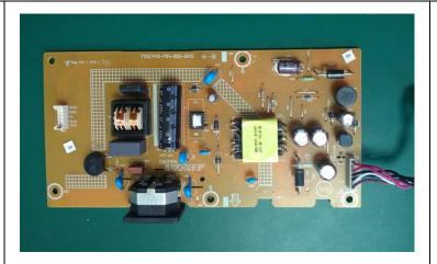
Remove electrolyte capacitors (red mark) from printed circuit boards
