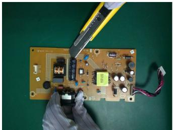
Lift the bulk cap. up and away from the PCB
