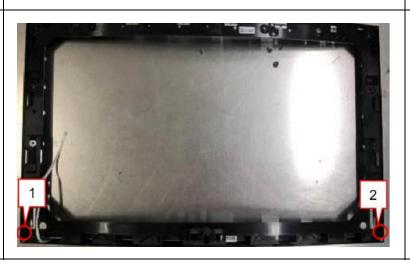
Use a Philips-head screwdriver to remove 2 screws for unlocking the key board (No.1~2 screw size=Q2x2.5.
