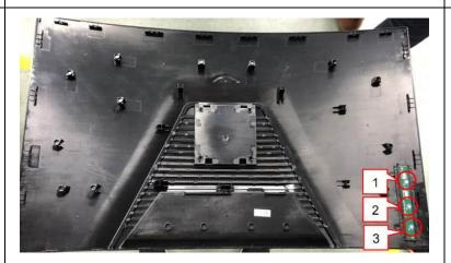
Use a Philips-head screwdriver to remove 3 screws for unlocking the key board (No.1~3 screw size=Q2x2.5, Torque=0.9±0.4kgf.cm)
