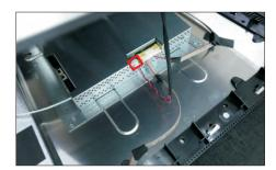
Use a Philips-head screwdriver to remove one screw for unlocking the USB board unit, then release the USB board unit and put it aside.
