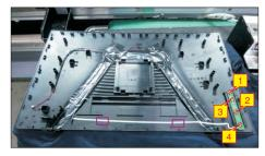
Tear off all the mylar and tapes, then use a Philipshead screwdriver to remove 7pcs screws for releasing the diffuser, reflector and LGP.
