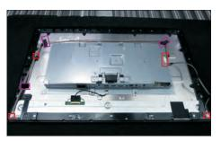
Tear off the mylar tape on the position as the picture below shown. Use a Philips-head screwdriver to remove 13pcs screws for unlocking the middle bezel with the panel module. Use a Philips-head screwdriver to remove 2pcs screws for unlocking the middle bezel with the front bezel.
