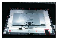
Remove the middle bezel and put it into a fixture jip, then use a Philips-head screwdriver to remove 1pcs screw for unlocking the power key board with the front bezel.
