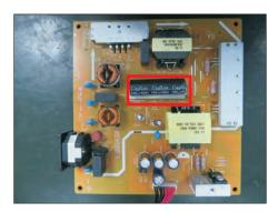
S19-1 Cut the glue between bulk cap. and PCB with a knife.
