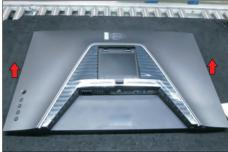
Lift the rear cover up carefully. Disconnect the USB FFC cable, joystick key cable and power key cable from the connectors of the interface board, and then disconnect the back LED light bar cable from the connector of the power board, and then remove the rear cover.
