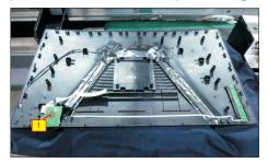
Use a Philips-head screwdriver to remove 4pcs screws for unlocking the joystick key board with the rear cover. Tear off the joystick key tapes and release the joystick key board from the hook of the rear cover.
