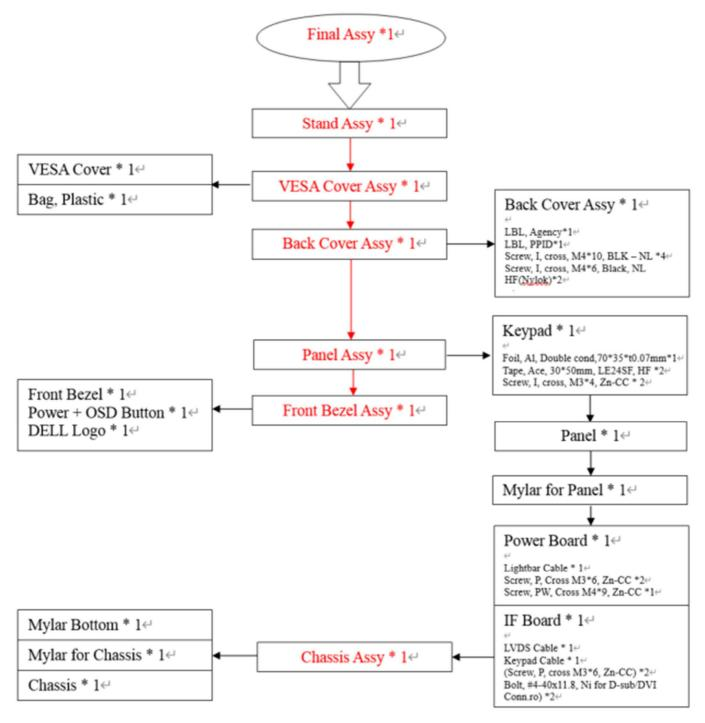
Note: 1. The arrows point out the direction of disassembly.
