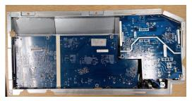
\$28 Disassemble wires from I/F BD
