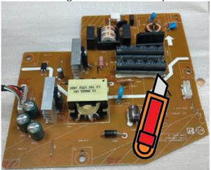
S31-2 Ensure cutting path within the glue, don't touch bulk cap. or PCB
