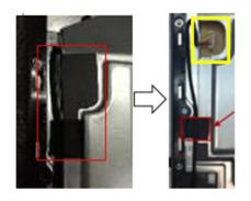
S15 Unplug "Power LENS FFC cable" from I/F BD and tear off "Power LENS FFC cable" from the panel
