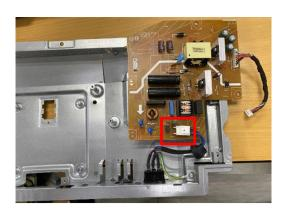
S30 Unlock 1 ground screw and disassemble AC power socket from Main SHD
