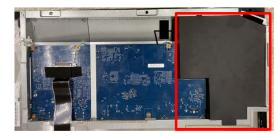
Tear off the adhesive tape on "FFC EDP" and unplug "FFC EDP " from I/F BD, then, Unlock 8 PCBA screws
