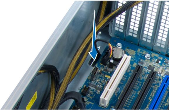
5. Remove the screws that secure the hard-drive fan to the computer chassis and remove the fan from the computer.
