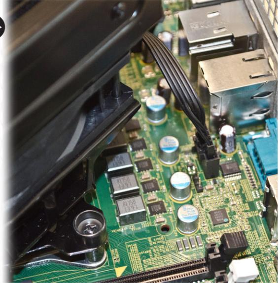
5. Press firmly on the heatsink and rotate clockwise.
