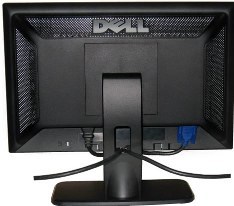
After attaching all necessary cables to your monitor and computer, (See [Connecting Your Monitor](#) for cable attachment,) use the cable holder to neatly organize all cables as shown above.
