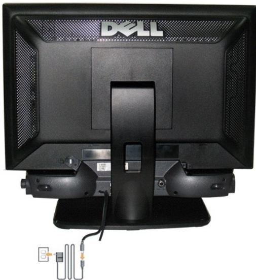
1. Working from the rear of the monitor, attach the Soundbar aligning the two slots with the two tabs along the bottom rear of the monitor.
