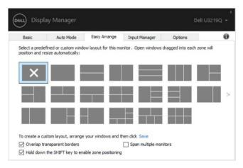
If you are using multiple monitors in an array or matrix, **Easy Arrange** layout can be applied across to all the monitors as one desktop. Select "**Span multiple monitors**" to enable this feature. You need to align your monitors properly to make it effective.
