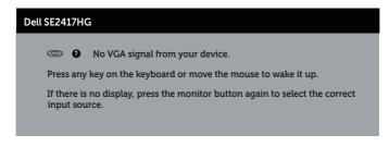
If VGA or HDMI cable is not connected, a floating dialog box as shown below appears. The monitor will enter Power Save Mode after 5 minutes if left at this state.
