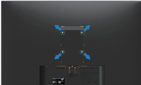
**NOTE:** For use only with UL-listed wall-mount bracket with minimum weight/load bearing capacity of 30.32 kg.
